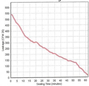
Your Heating and Cooling Capacity Improvement for Duct Sealing is 23%
